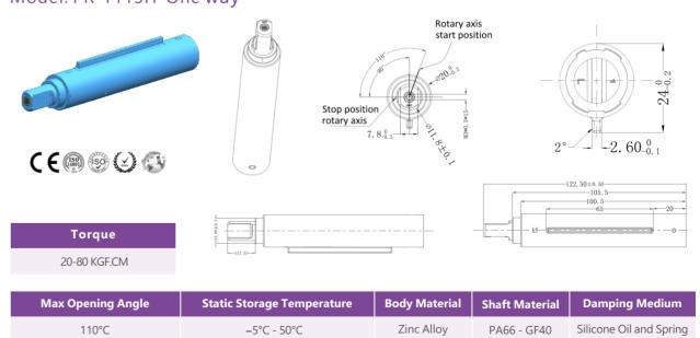
Remarks: For T115 series dampers can also apply in high temperature environment(up to 120 degree), by using heat-resisting material. Such as in cooking ranges, ovens, etc.
