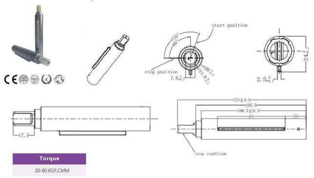
Remarks: For T115 series dampers can also apply in high temperature environment (up to 120 degree), by using heat-resisting material. Such as in cooking ranges, ovens, etc.
